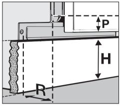
The panel overhang (**P**), and toekick depth of recess (**R**), determine the maximum dishwasher toekick height (**H**).
